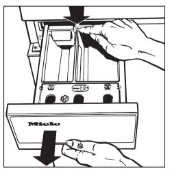
■ Press down the red release lever and pull the drawer out of the machine.
